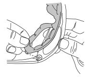
Align one outside gasket tab to the frame slot, while holding down with your finger, press the top of the gasket down until the inner tab clicks into the slot near the nose bridge. Repeat on the other side.
