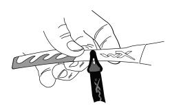
Align the plastic T-Peg as shown and press into temple arm. The strap is locked into place when the plastic T-Peg is rotated back and parallel to the frame. To remove, rotate the plastic T-Peg perpendicular to the arm and pull out. MAINTENANCE: Wiley X lenses are specially coated to offer superior abrasion resistance. Please follow below instructions to prolong the life of your lenses and keep them performing at their best:
